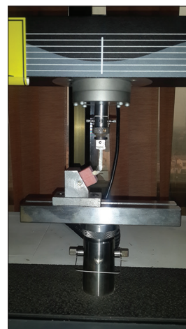
Figure 3: Loading of the tooth at 60° angle
