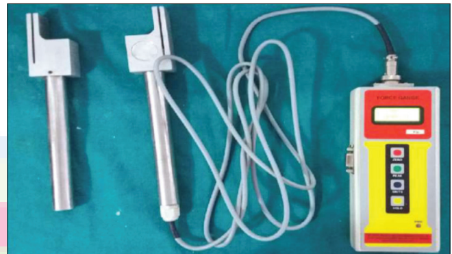
Figure 20: Transducer bite force measurement device with analog for bite equalization
