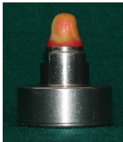
Figure 2: Wax pattern on master die
