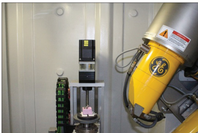
Figure 5: Master die placed in the micro-computed tomography scanner
