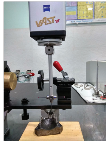
Figure 12: Transfer coping screwed in implant analog for interimplant distance measurement
