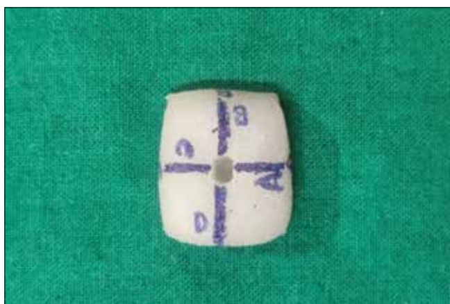
Figure 1: Customized acrylic die with markings of (A-D)
